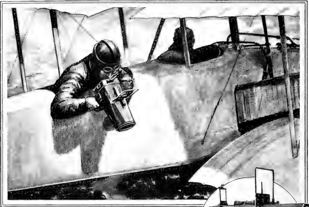
The Photographer in His Aeroplane Can Point the Pistol-Camera with Great Accuracy at the Object To Be Photographed. The Two Focusing Frames Take the Place of Sights on a Revolver. The Trigger Operates the Shutter
